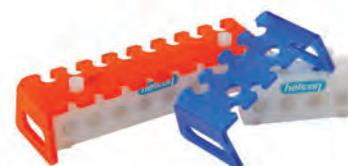
Rack of the «Polyus» series, designed for individual test tubes, consist of two modules an upper removable test tube rack-holder and the magnet itself, making it possible to move the test tubes placed in rack without moving the magnet.
